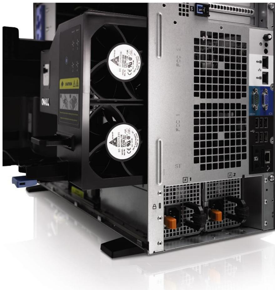
Figure 5. Fans and Cooling Shroud
