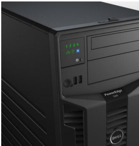
**Figure 10. LED Control Panel**
