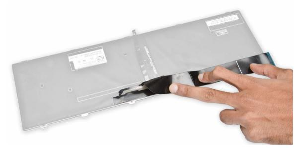
**3.** Gently fold the keyboard-backlight cable at the fold line.
