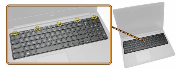
8. Press the locations indicated in the picture to complete the keyboard installation.
