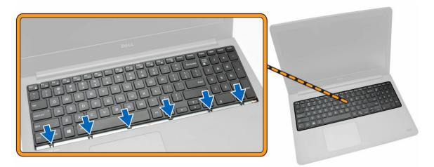
7. Press on the sides of the keyboard followed by the locations marked in the picture to firmly seat it.
