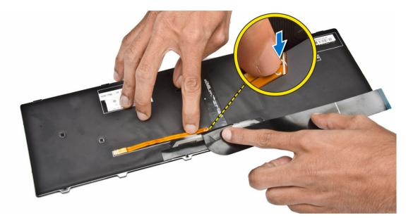
4. Place the keyboard-backlight cable underneath the keyboard connector cable as indicated.
