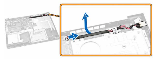
4. Remove the power connector from the computer.
