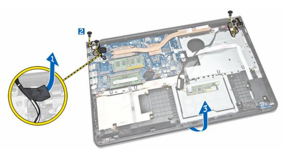
**4.** Lift up the base unit and slide it out.
