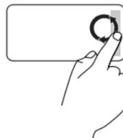
Move a finger in the vertical scroll zone (extreme right of the touch pad), in a clockwise circular motion to scroll up or counterclockwise circular motion to scroll down.
