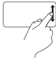
Move a finger up or down in the vertical scroll zone (extreme right of the touch pad).
