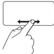
Move a finger right or left in the horizontal scroll zone (extreme bottom of the touch pad).
