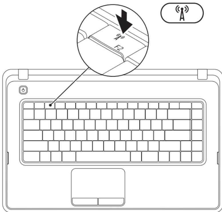
Press the **Fn** key on the function key row on the keyboard to enable or disable wireless. The wireless on or off icons appear on the screen to indicate the status.
