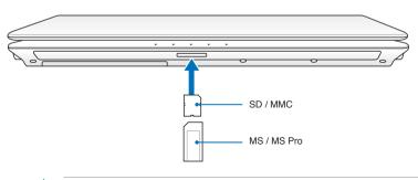
The actual location of the Flash Memory Slot differs by models. Refer to the previous chapter to locate the Flash Memory Slot.
