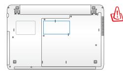
WARNING! Disconnect all the connected peripherals, any telephone or telecommunication lines and power connector (such as external power supply, battery pack, etc.) before installing or removing a memory.
