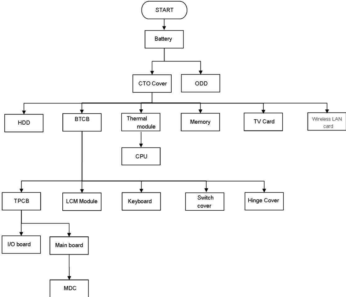
**LCM module disassembly flow chart**
