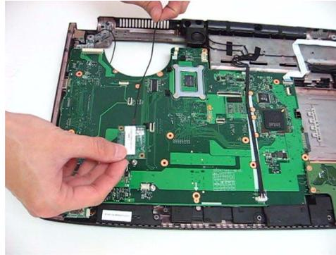
18. Disconnect Speaker cable from the MB and loose the MB screw.
